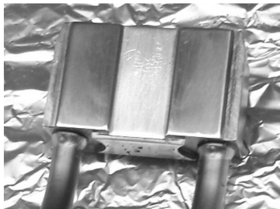
Figure 19: HP West's X-ray anode after a fine sandpaper and rubber eraser scrub.
